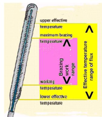
Fluxes applicable for the brazing with Silver-Copper-Zinc alloys are the type FH10 acc. to EN1045 (previously F-SH 1 acc. to DIN 8511) with operation temperatures of 550-800°C used for Silver alloys. For silver-free alloys a flux FH21 or FH20 with a temperature range of 750-1000°C is recommended.
