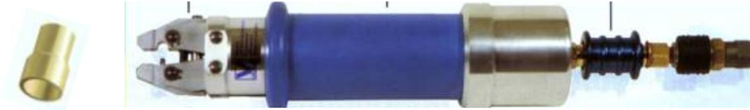
First the pneumatic tool is crimping the tool, then some glue is applied to tube end and the stopper on the tube positioned on tube end by turning. Afterwards the tool is placed on the Lockring stopper to seal the tube. By opening of the sliding valve the Lockring is pressed over the collar of the stopper and the tube end is sealed.
