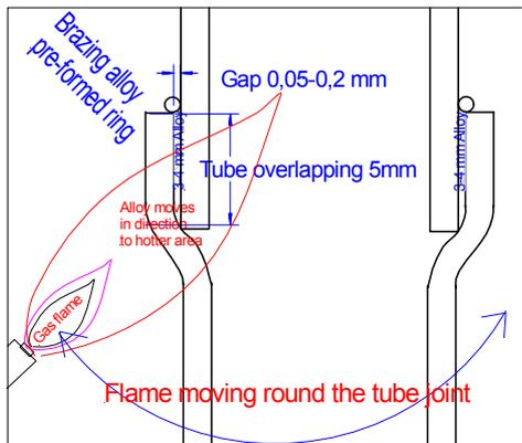
De-burred “Broken corners” at the beginning and end of a capillary path will enhance filling of the joint. At least burrs must be removed. Never incorporate a groove midway through a joint (unless used for placing a brazing alloy ring to be heated).
