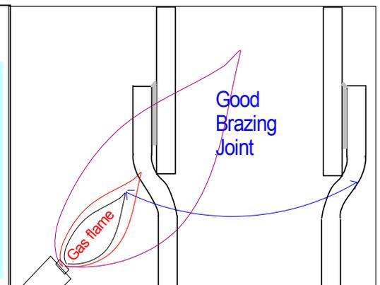
Furthermore we recommend using **compressors with copper coated steel tube ends** easier to braze as the ones without such coating. But copper coated steel tubes have to be treated in brazing as steel tubes, not copper tube joints.
