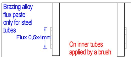
To joint **overlapping** steel tubes the simplest and safe solution is the application of a flux paste in the correct temperature ranges FH10 for Silver alloys or FH20 or FH21 for silver free alloys. With a small brush (4mm width) the paste can be painted around the outer surface of the inner tube with a layer of about 0.5-1 mm thickness, at least 0.2 mm layer. This should be done at the position on the assembly line in which the tubes were assembled and not at the brazing position.
