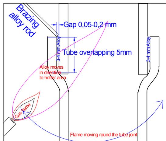
The problem is that a flame (especially if Oxygen is added) surely will more rapidly heat up exterior surfaces as interior joints. To reach a more balance heat pattern the parent metal must have time to conduct the heat away from the flame application points to the interior parts. It should neither be **over-heated** which would cause
