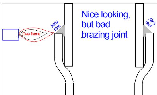
Typical for such an application is the nice **fillet** above the tube gap - quality inspectors like it, as they can see the seal -, while a correct sealing of overlapping tubes with low quantity of alloy can only be inspected by destroying the joint or X-ray. Such a bad fillet seals the tube joints, but can break under stress and on longer time.
