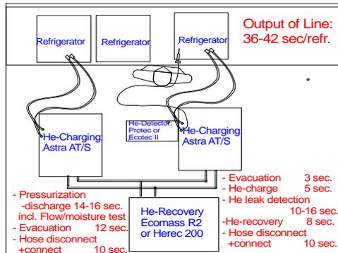
**a) 2 Helium, dry air and Nitrogen charging boards on same line with 1 operator and 1 leak detector**
