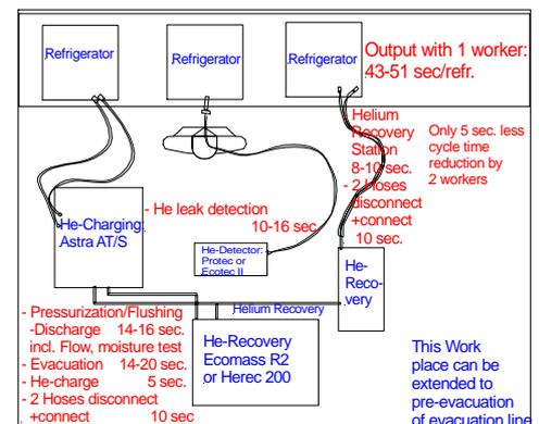
The Helium leak detection after final assembly and brazing of the cooling circuit are followed by the evacuation process, today done in 2 stages: pre-evacuation 60-120 min., waiting time of 6-8 min. and final evacuation of 15 min. Therefore it is useful to combine the Helium recovery with the pre-evacuation to an automatic station with red and green signal lamps to remove Hansen connections when it is finished and reconnected it to next refrigerators for Helium recovery and pre-evacuation.
