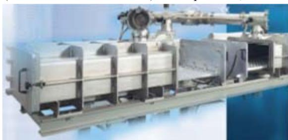
The component is pressurized with Helium and a built-in Helium leak detector **Inficon UL200** is connected to the chamber to measure total leak. The system also allows executing pressure test at 30 or even 40 bar
