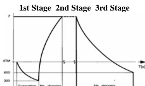
The **total cycle time of the first stage is min. 32 s up to 44 s**, if more evacuation is wished to reduce Helium consumption (The fixing of the 2 quick coupler male Hansen tube squeezing adapter on the refrigerator is not yet added to the cycle time).
