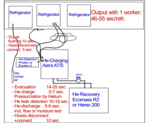
To avoid humidity inside the Helium in case drying failed, a filter dryer should be added and the filter insert regularly exchanged by a dry one.
