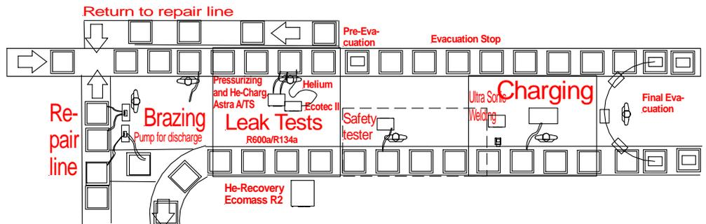
The ultrasonic welding could be made together with the refrigerant charging and the pre-evacuation together with safety test.
