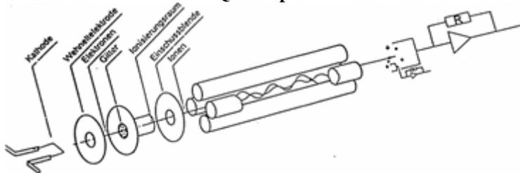
The HQ200 mass spectrometer as built in the Ecotec consists of an ion source, a quadruple mass filter and an ion detector (see assemblies in figure on left). The figure underneath schematically shows the pattern of the electrical potential. The ionization chamber is formed by a grid and the subsequent cylinder. It is connected to approx. +150V relative to ground. The iridium cathode coated with thorium oxide is connected to approx. +50 V relative to ground.
