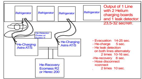
This is an optimal solution for investment and work cost: either to be done on 2 parallel lines (version b)) or to be done on one fast line (version c) with 2 Astra III and only 1 Helium leak detector by 1 operator. But let us see if other remaining theoretical solutions provide improvements concerning utilisation of investment or work.
