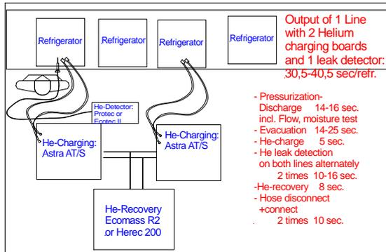
**c) 2 Helium Charging board with 1 worker and 1 Helium leak detector**
