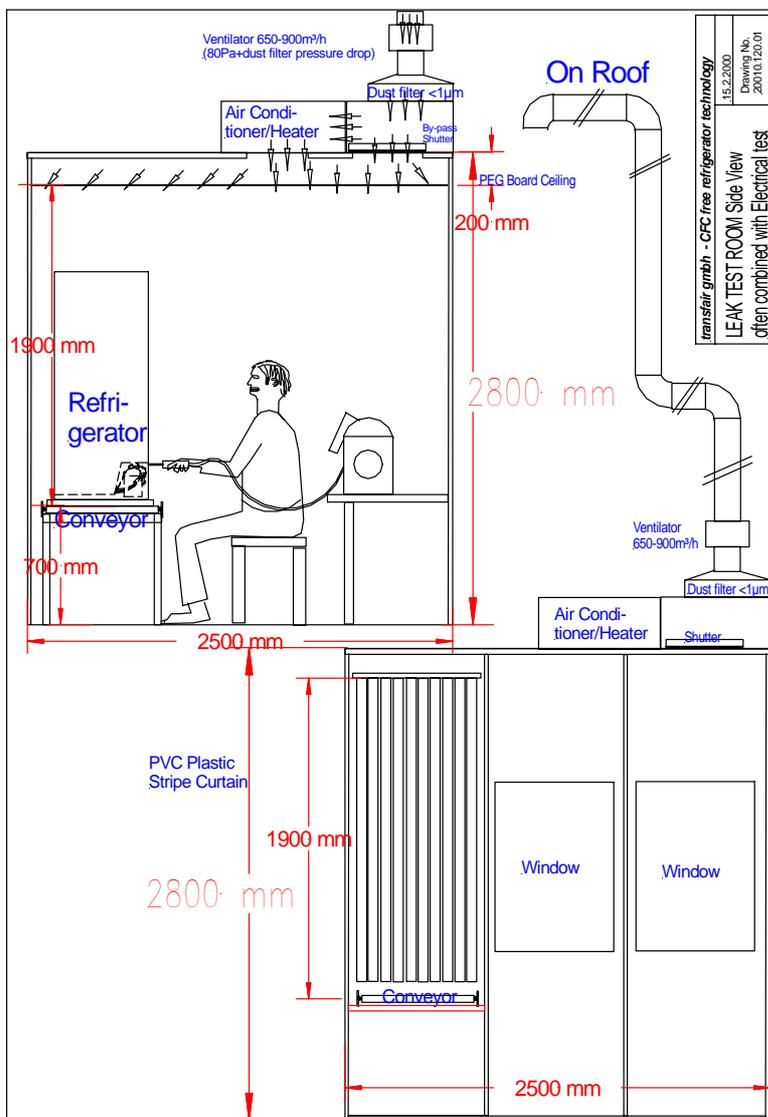
**Electricity.** There exist 3 different Voltages versions (220-230V, 100-120V, 127V) 1Ph, N, PE, underneath 400VA, internal fuse of 2.5A, for a.m. mass spectrometric leak detector with +10/-15% deviation tolerance. The major needs concern the a.m. ventilation and air conditioning depending from the local conditions.
