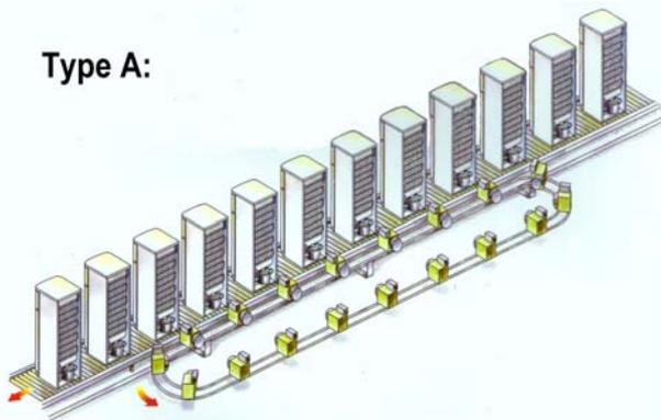
Type A is the less economic way, which needs nearly doubles as much pumps as the Type B and C. If the pre-evacuation (about 1-2 min.) and the evacuation interruption of 6-8 min. is done before the carousel about 30% less pumps are needed.
