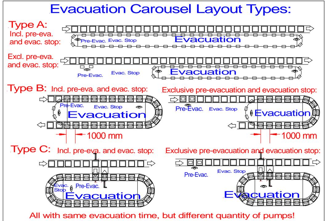
have pumps on ground or above the refrigerators in high:
