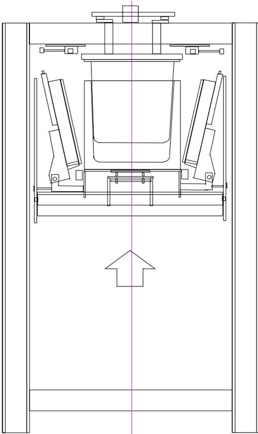
How these tolerances can be absorbed and how at the end we receive a correct manufactured and dimensioned refrigerator? The trick is the foaming during which all parts are correct positioned and with the foam fixed.
