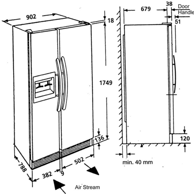
**Dimensions for a typical side by side refrigerator-freezer combination**
