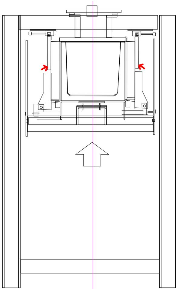
**2<sup>nd</sup> Phase: Adjustment of side panels to liner by turning the side support and closing into the upper lock profile.**
