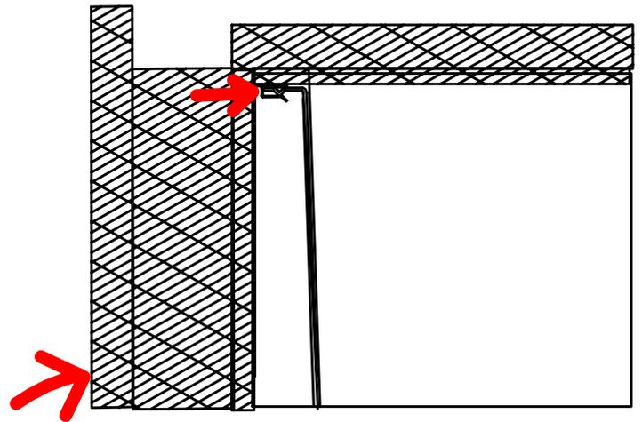
At this stage the 2 side panels are parallel, but still one panel could be nearer to the top support as the other one. The 3<sup>rd</sup> phase adjust it by turning the bottom and
